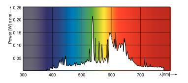
Spectral Power Distribution Colour - MC CDM-R Elite 70W/930 E27 PAR30L 40D
